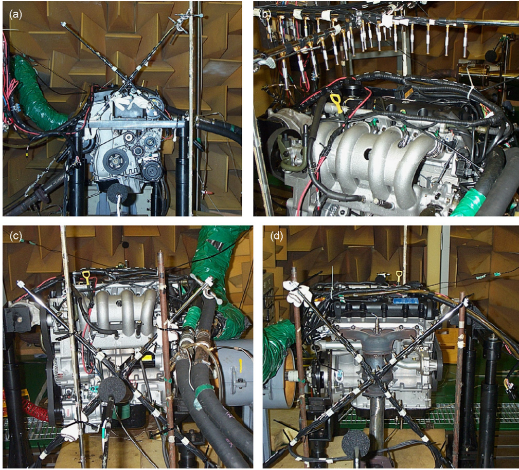
Fig. 6. The experimental setup for the automobile engine to identify the impulse noise source. Sampling frequency is 32.8 kHz, the number of microphones is 28 and the total length of time is 5.5 s: (a) Front side, (b) upper side, (c) right-hand side, and (d) left-hand side of the engine.
